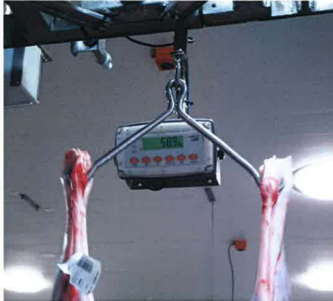
The cold weight is recorded as the carcass is moved to the boning room Boning rail - shows skid EID readers and load cells (weighing)
