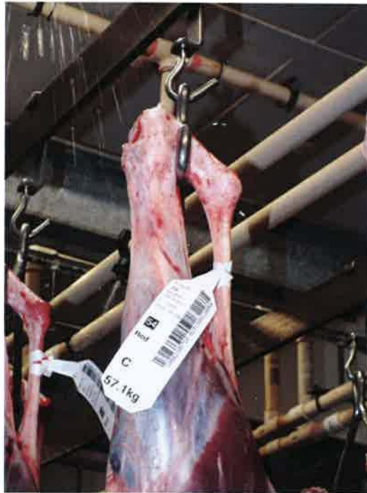
Printed carcass ticket with electronic information as a back-up to the electronic identification The photo also illustrates the fine spray in the chiller.
