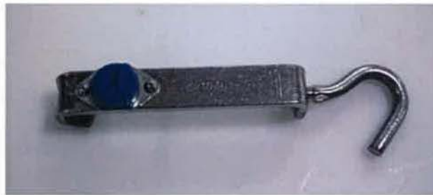
Carcass skid which follows the carcass throughout the slaughter and boning process
