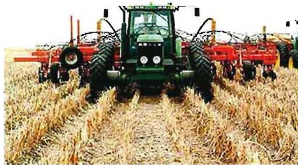
Figure 2 Modified tractor used in controlled traffic farming
