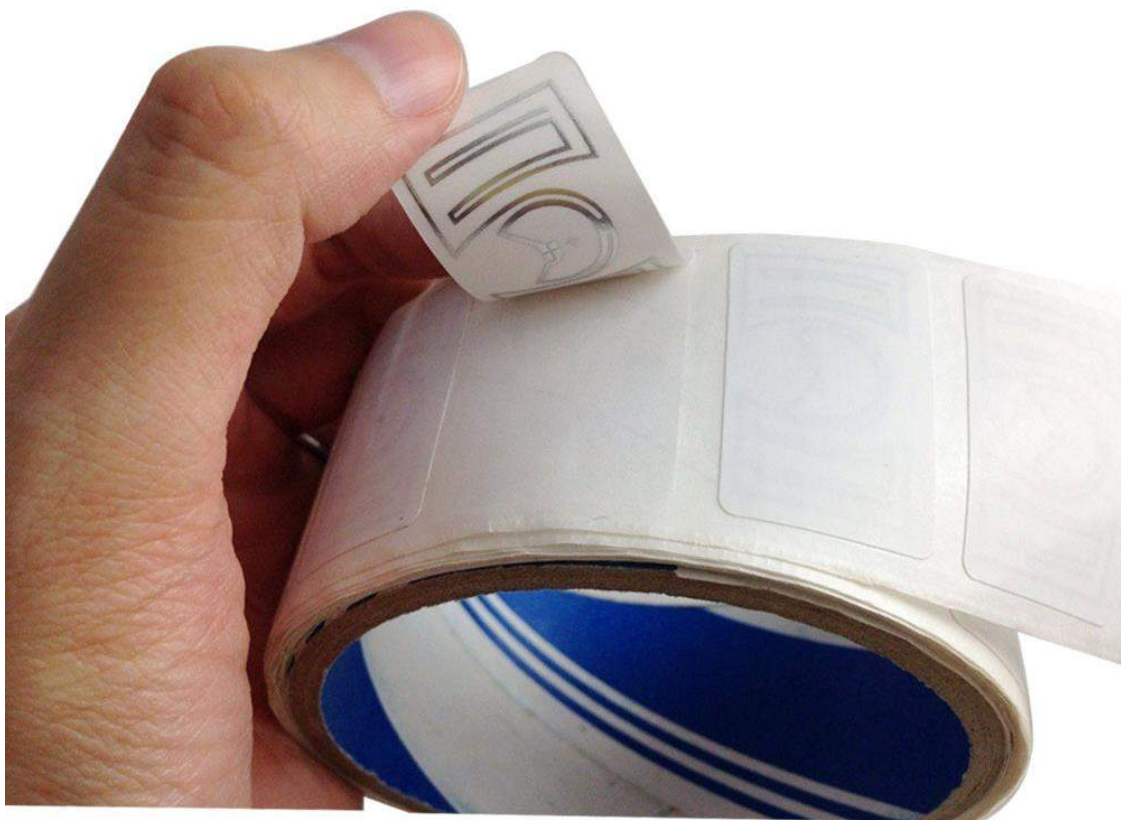
Figure 11: A RFID sticker being peeled off a roll from Produmex (2015).
