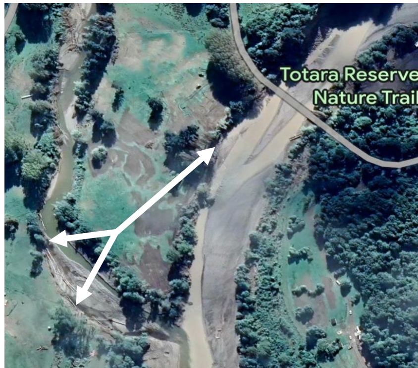
Figure 6 Arrows pointing to bends in the river channel susceptible to erosion caused by flooding. These are beneficial areas for groyne construction to avoid further erosion, productive land loss and to protect fragile infrastructure close by (Modified from Google Maps, 2023).
