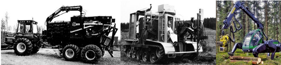
Figure 15. Examples of significant investment in technology that either was never, or is no longer, operationalised: The Silva Nova (left), ReForester prototype automatic injection planting machine (middle), and the PlusJack (walking harvester) (right).
