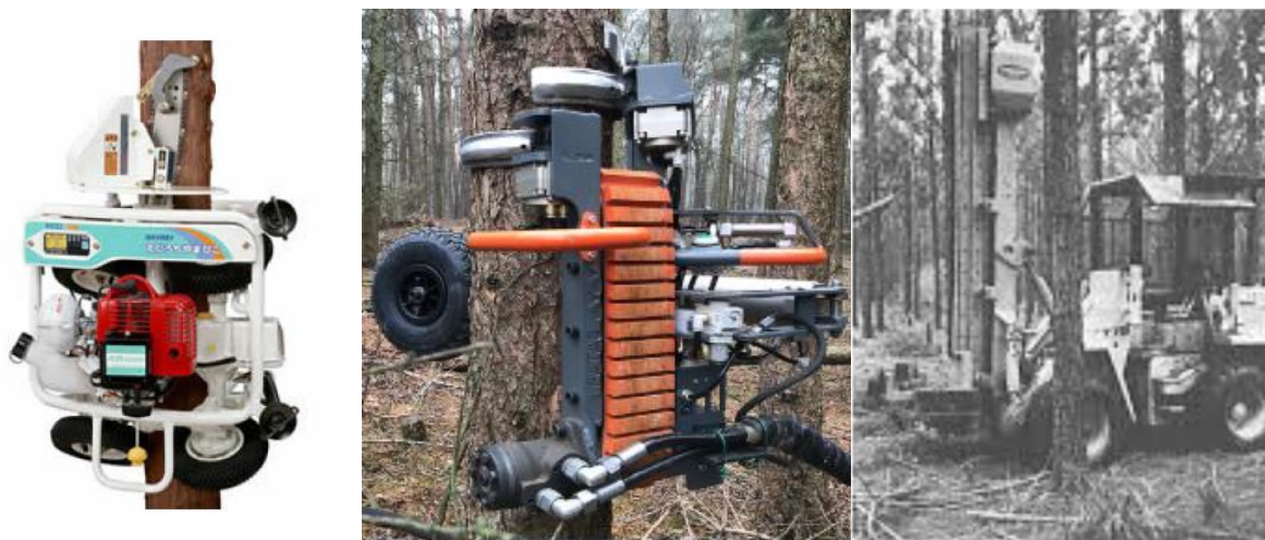
Figure 6. Mechanised pruning machines. The 'YAMABIKO' (left), the 'Patas' (middle), and the 'Paterson Pruner' (right).
