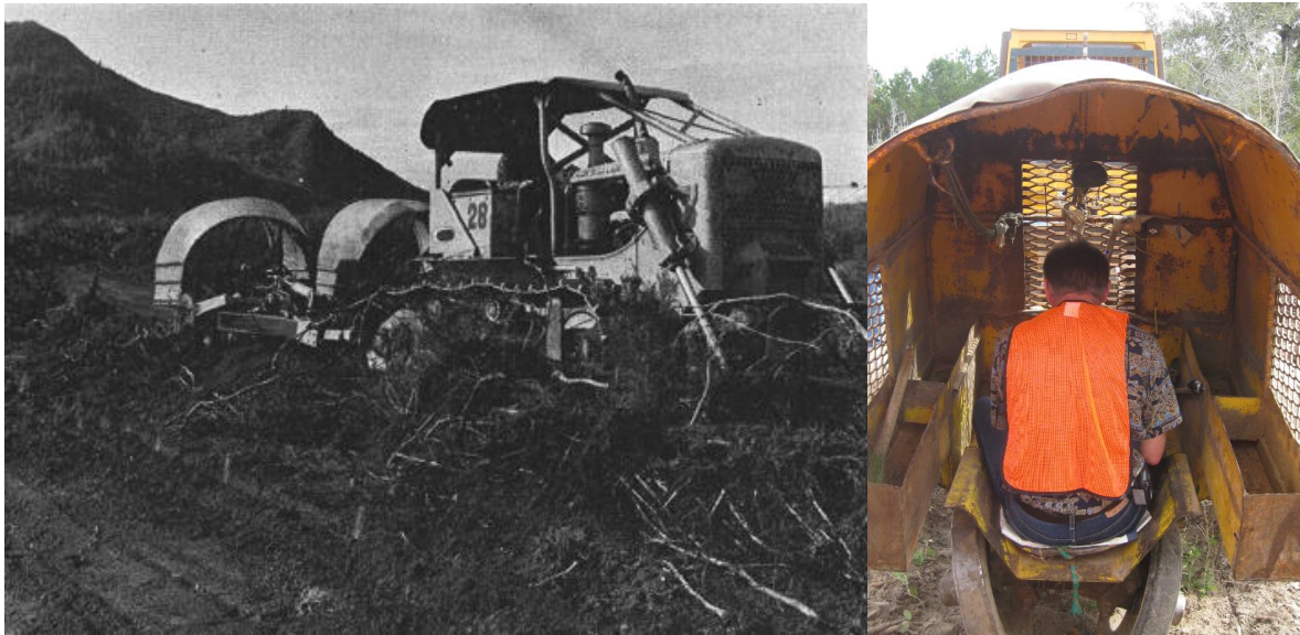
Figure 1. Double unit Lowther planters hauled by a crawler tractor, Tarawera forest, 1960s (left). Rear view of similar planting machine in USA (right)
