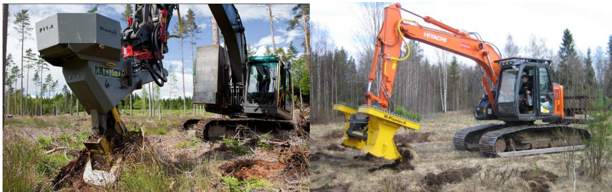
Figure 3. Modern planting heads on excavators. The Bracke tree planter from Sweden (left) and the M-Planter from Finland (right)
