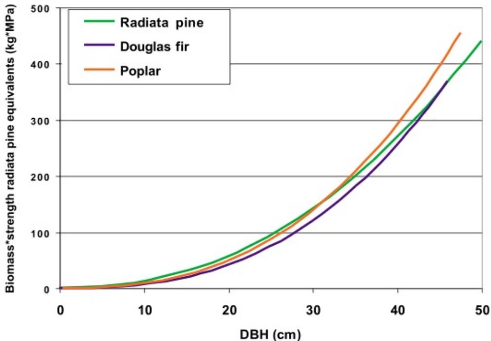
Figure 8: Root Biomass multiplied by tensile strength relative to Radiata (Knowles. L, Feb 2006)
